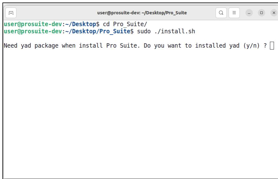
Figure 2-3 Install yad package
